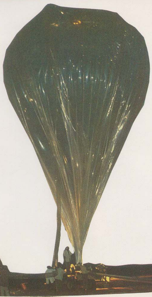
Hydrogen inflated balloon ready for launch at the National Balloon Facility in Hyderabad to study middle atmospheric parameters
