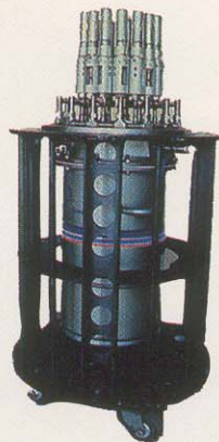
Balloon-borne cryogenic air sampler
