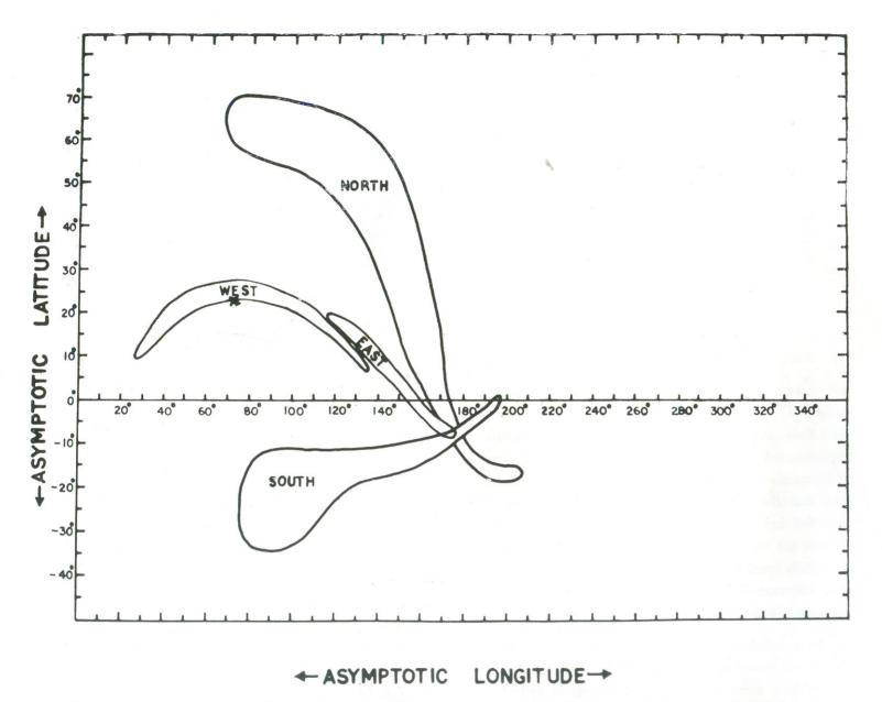
Directions in space from which cosmic ray particles reach the various inclined meson telescopes at Ahmedabad
