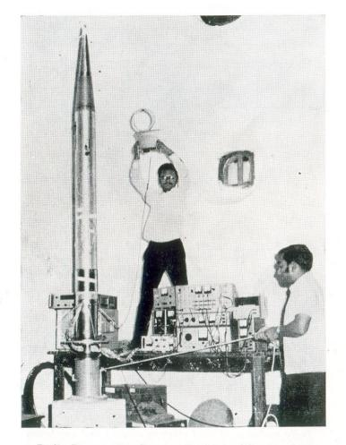
Radio Propagation Receiver Payload calibration during shock test
