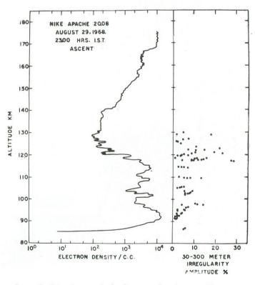
Irregularities in vertical electron density profile using a rocket payload
