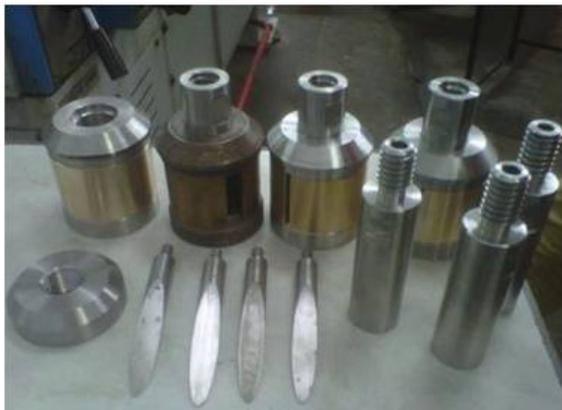
Figure 104: Various tools developed at PRL Workshop for underwater coral driller.
