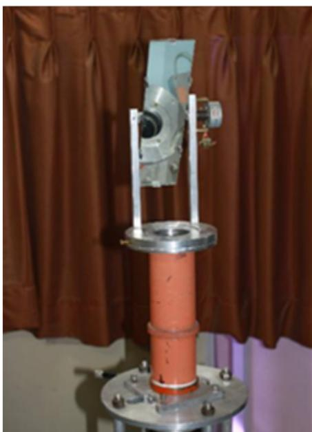
Figure 99: Mirror scanner for air-glow spectrometer.
