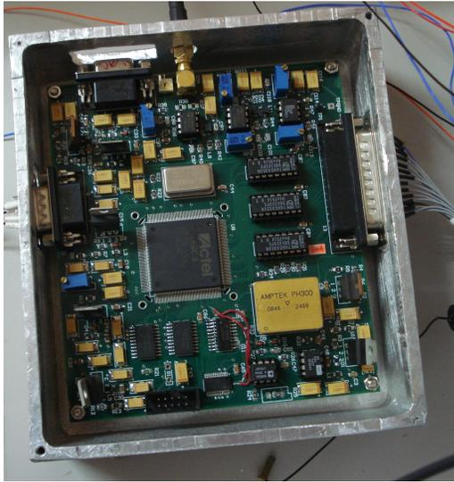
Figure 62: Bread-board model of GRS electronics developed in PRL combining shaping and processing electronics within a single PCB.
