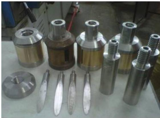
Figure 103: Various tools developed at PRL Workshop for underwater coral driller.
