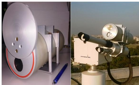
Figure 4: Spectral Sun photometer (left) and photometer mounted on Sun tracker (right).
