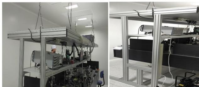
Figure 6: Tables using Aluminium profiles for optics laboratory.
