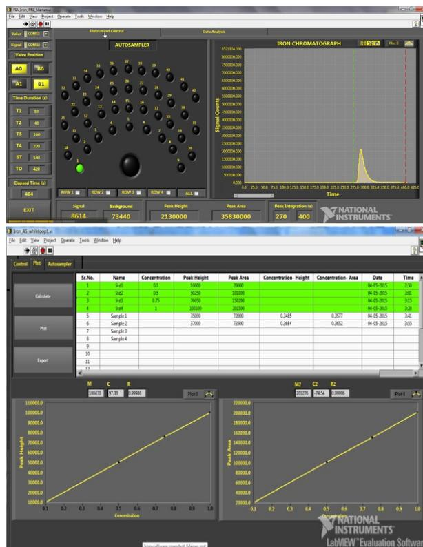
Figure 2 : Typical chromatogram of Fe (top) and calibration graphs for both peak height and peak area (bottom).
