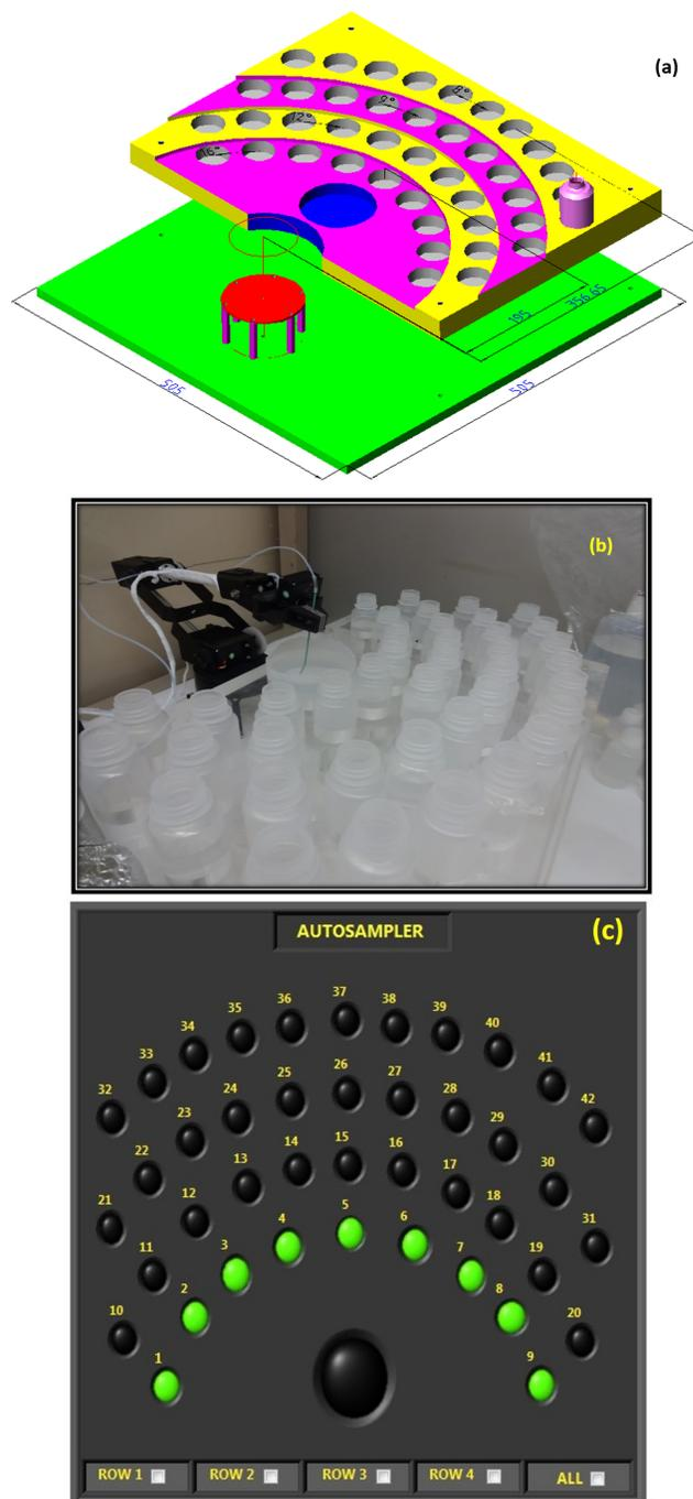
Figure 24 : (a) Autosampler Structure (3D), (b) Autosampler with Robotic Arm and (c) Software User Interface for control.
