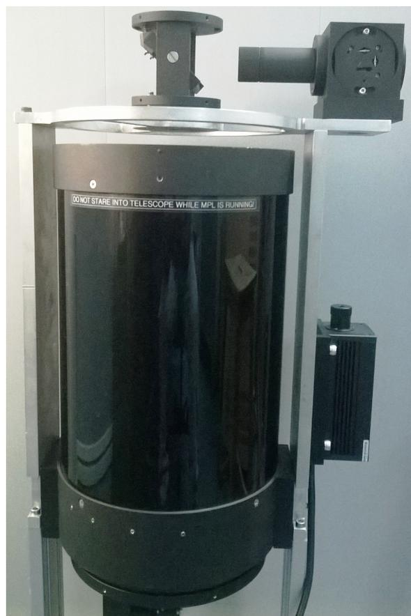
Figure 3: Portable micro pulse Lidar.
