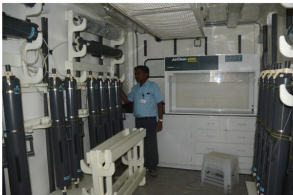
Figure 2: Clean van with Niskin sampling bottles.
