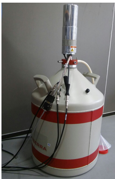
Figure 37: HPGe detector with 30 ltr \text{LN}_2 dewar
