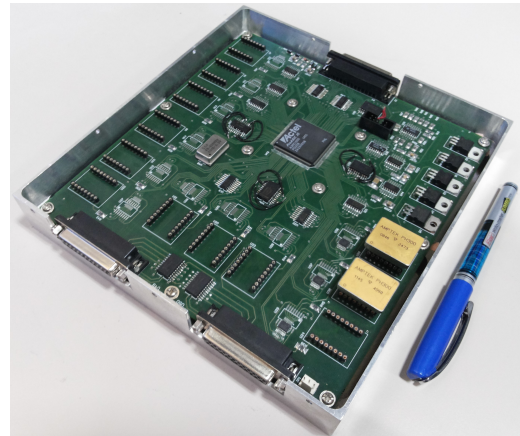
Figure 35: PCB for STEPS processing electronics (PCB size 220 \times 220 \text{ mm}^2 )
