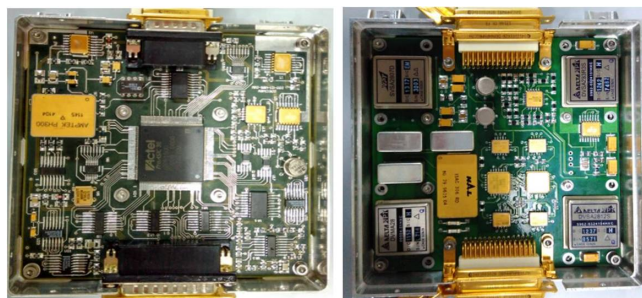
Figure 23: Photographic view of XSM processing electronics package, FPGA (left), DC-DC converter (right)
