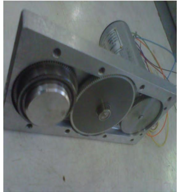
Figure 2: Optical element coupling unit of an imaging polarimeter for 1.2 m telescope at Mt Abu Observatory. The fully assembled coupling unit is shown in the left and the gear box on the right.
