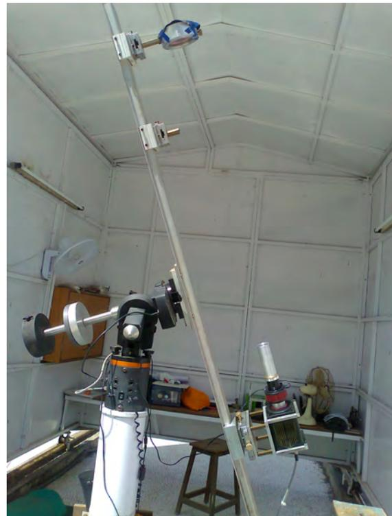
Figure 12: Thaltej Solar Flare Telescope of Physical Research Laboratory operating at Thaltej campus. The 10-cm aperture refractor with  $f/16$  focal ratio provides 13 mm image at prime focus. The quantum  $H_2$  filter copuled with CCD provides images with a cadence between 10ms to 5s as desired.
