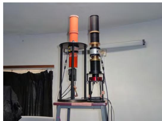
Figure 3: The fully assembled airglow photometers, fabricated in PRL workshop.
