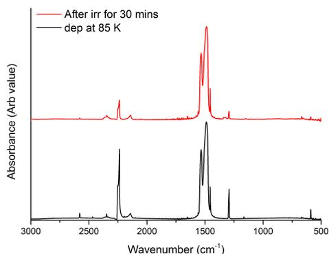
Figure 2: Infrared spectra of  $CS_2$   $N_2O$  ice mixture after deposition at 85 K (black) and spectra after irradiating the ice mixture for 30 minutes (red).
