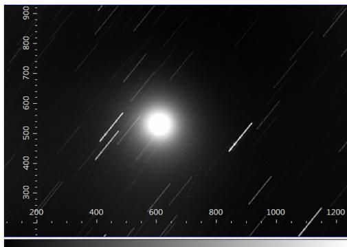
24.12.2014, UT: 18:47:06. The comet imaged at sloan g'2 band (400nm-550nm) wavelength, also the spectrum captured using star analyzer grating (SA-100) within filter wheel fixed with 0.2m SCT telescope mounted on sky-watcher NEQ6 mount.
