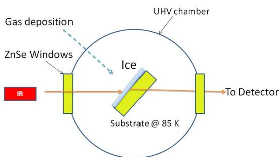
Figure 1: Schematic of the Experimental setup housed at PRL, Ahmedabad used to record the Infrared spectra of Astrochemical ices containing a Zinc Selenide ( $\text{ZnSe}$ ) substrate cooled to 85 K in an Ultrahigh Vacuum chamber with a pressure less than  $10^{-9}$  torr.
