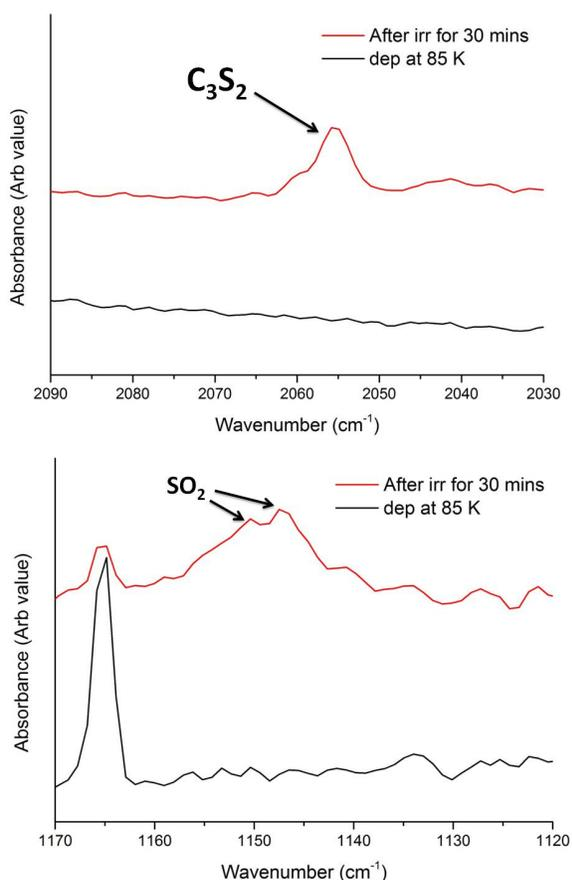
Figure 3: Infrared spectra of the ice mixture before and after irradiation (a)  $C_3S_2$  observed after irradiation at  $2055\text{ cm}^{-1}$  and (b)  $SO_2$  after irradiation at  $1150$  and  $1154\text{ cm}^{-1}$
