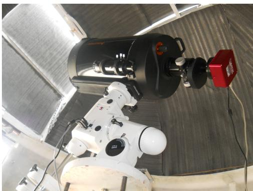
The spectral image captured over sensor KAF8300 (Atik383L+ cooled monochrome CCD) coupled with filter wheel assembly. The comet image manually guided over the field of view of CCD using double cross view application of APT- Astro Photography Tool. The telescope mount was commanded using EQ-direct (ASCOM platform supported) + Starrynight (SN7). The 50 images are stacked in maximDL and false color image created in DS9. The spectral image files processed in RSpec spectroscopy software.
