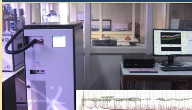
**Figure 2:** Measurements of monoterpenes ( $\alpha$ -pinene) and other VOCs using high mass- and time- resolution PTR-TOF-MS instrument at PRL, Ahmedabad.
