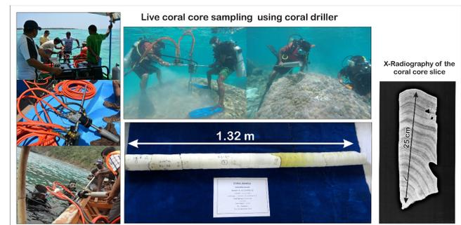
Figure 15 : Demonstration of the underwater coral driller in operation. Coral core section recovered from the Lakshadweep Islands and X-Ray section of the sample showing annual bands.
