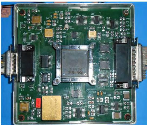
Figure 41b: Photograph of XSM processing electronics subsystem
