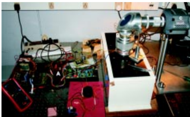
Fig. 54: A view of the spatially resolved Luminescence System developed at PRL A) Control Electronics B) Stimulation assembly and optical arrangement C) CCD Camera.
