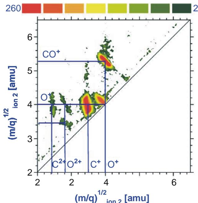
Fig. 6.8 The covariance map of ion pairs formed by photo-fragmentation of  $\text{CO}_2$  molecule by 200 eV photons, showing  $[\text{O}^+:\text{CO}^+]$ ,  $[\text{C}^+:\text{O}^+]$ ,  $[\text{O}^+:\text{O}^+]$ ,  $[\text{O}_2^+:\text{O}^+]$ ,  $[\text{O}_2^+:\text{C}^+]$  and  $[\text{C}_2^+:\text{O}^+]$  coincidences.
