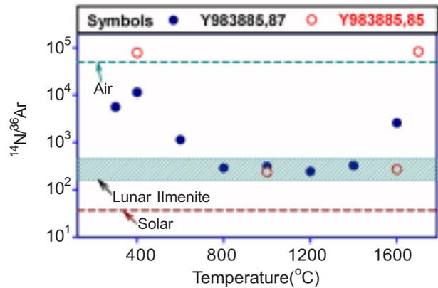
Fig. 7.2 Release pattern of  $^{14}\text{N}/^{36}\text{Ar}$  ratio in two samples of lunar meteorite Y983885.  $^{14}\text{N}/^{36}\text{Ar}$  value of Air, solar component as well as the range observed for lunar soils are also shown in the plot.
