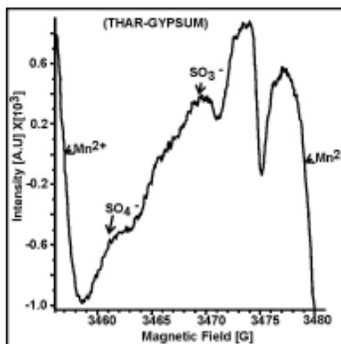
Fig. 7.3 A typical Electron Spin resonance spectrum of Gypsum.
