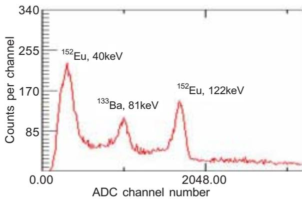
Fig. 8.2 Spectra recorded by one CZT pixel and PRL FEE using the gamma sources  $^{152}\text{Eu}$  and  $^{133}\text{Ba}$ .
