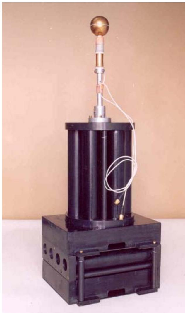
*A Langmuir Probe and Photometer Assembly fabricated at workshop for measuring Electron Density and studying Nightglow Emissions for rocket borne payload, ABHA. The work of designing and modeling of Electronics Package Box has been completed by using software Mechanical Desk Top (MDT-6) and also fabricated at workshop.*
