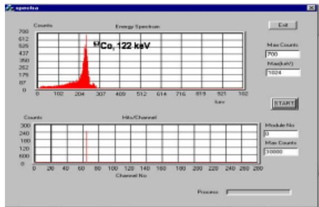
Fig. 8.3 Spectra recorded by a CZT pixel with PRL FEE and ground checkout system using the gamma source  $^{57}\text{Co}$ .
