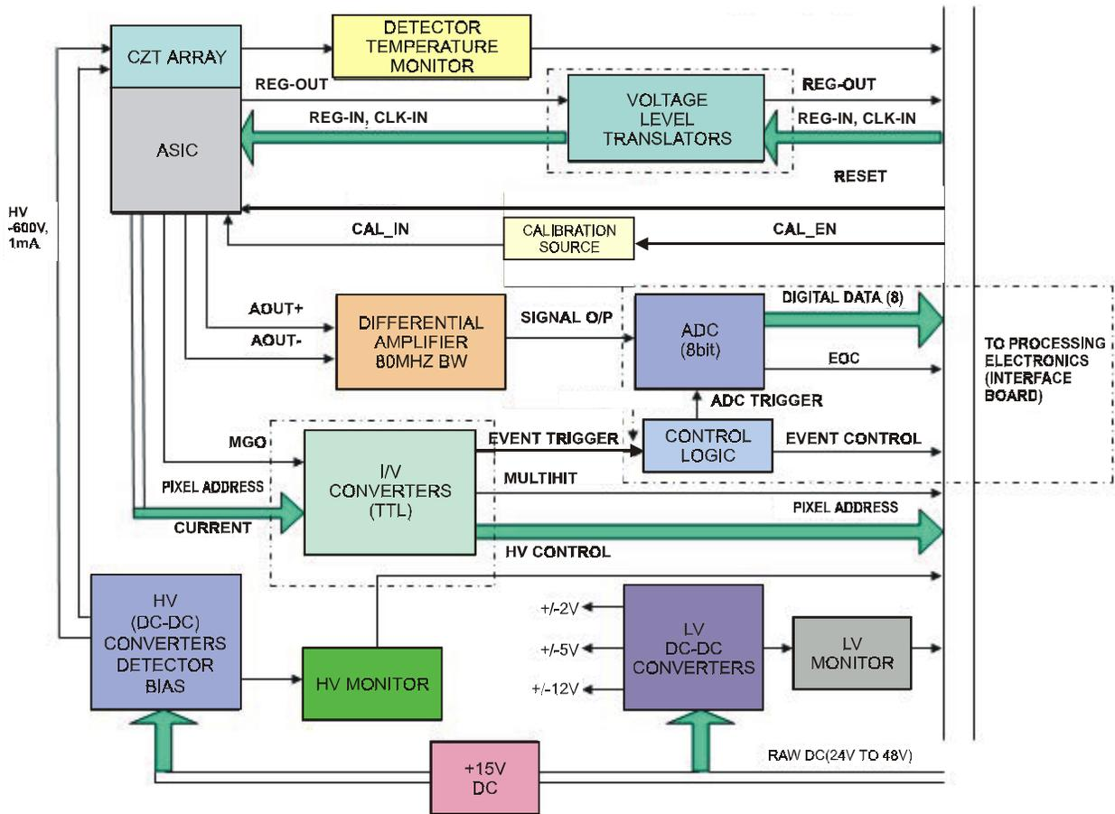
Fig. 8.1 Schematic diagram of front-end electronics for HEX payload.
