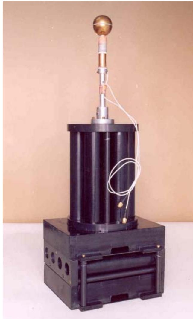
*A Langmuir Probe and Photometer Assembly fabricated at workshop for measuring Electron Density and studying Nightglow Emissions for rocket borne payload, ABHA. The work of designing and modeling of Electronics Package Box has been completed by using software Mechanical Desk Top (MDT-6) and also fabricated at workshop.*
