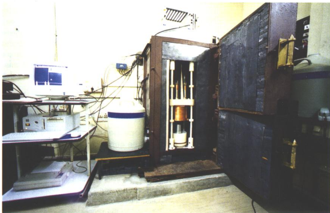
Fig.6.8 A specially built counting system for assaying the very low level radioactivity produced by cosmic rays in meteorites
