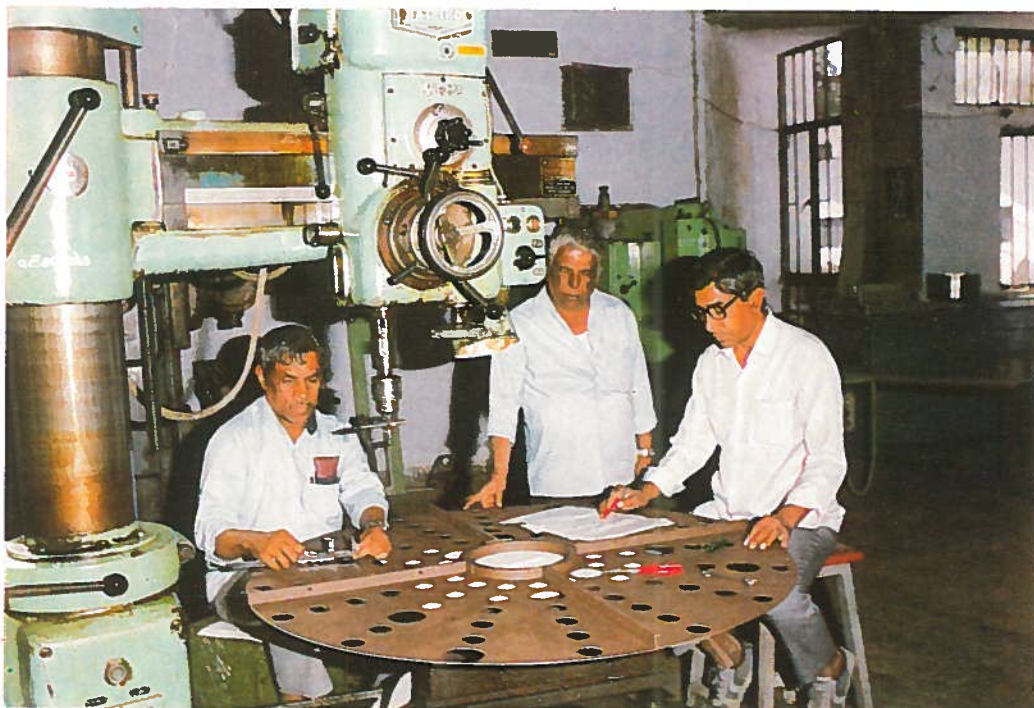
"Hartmann's Screen" under preparation on radial drilling machine. This screen will be utilised for testing the 48" diameter Mirror at Mt-Abu.
