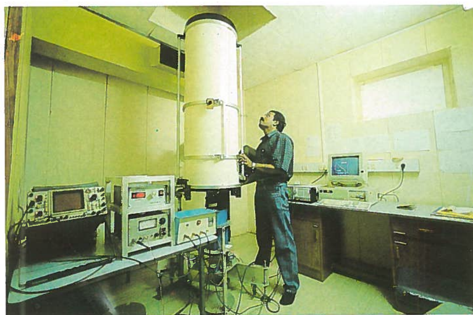
The Nd - YAG Lidar system at PRL for studies of atmospheric aerosols.
