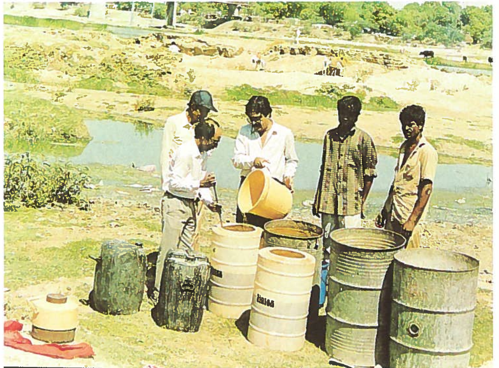
Tracer solution being prepared for tracer tests to see if there exists a rapid channel type flow between the sewage poll and the radial collector (French) well seen in the background.
