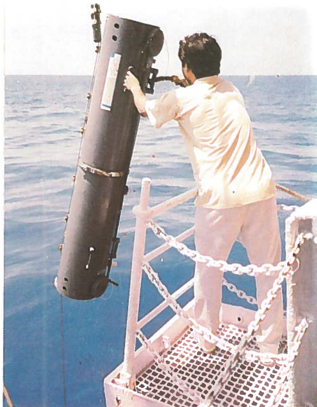
GoFlo Seawater Sampler ( capacity : 100 l ), used for ocean circulation studies using radiocarbon. (a) Empty sampler ready to go down and (b) sampler filled with seawater brought up from greater depths.
