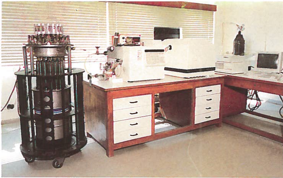
Photograph showing the GC-MS system together with the cryogenic air sampler. The sampler will be launched on a balloon to collect air samples at different heights.
