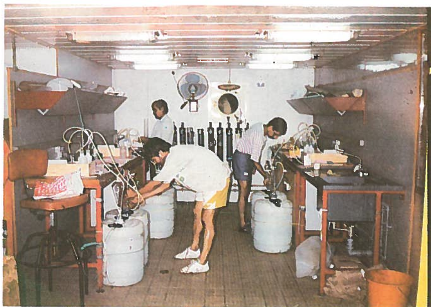
Laboratory in Research Vessel Sagar Sampada of the Dept. of Ocean Development, where \text{CO}_2 is recovered quantitatively from ~ 100 l water into 250 ml sodium hydroxide solution.
