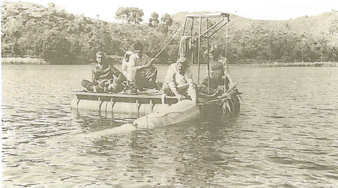
3 Meter Corer and a floating platform indigenously designed and fabricated in PRL Workshop is seen under operation at Mansar Lake near Jammu.
