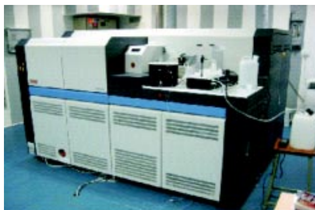
Fig. 29. The newly installed MC-ICP-MS at PRL
