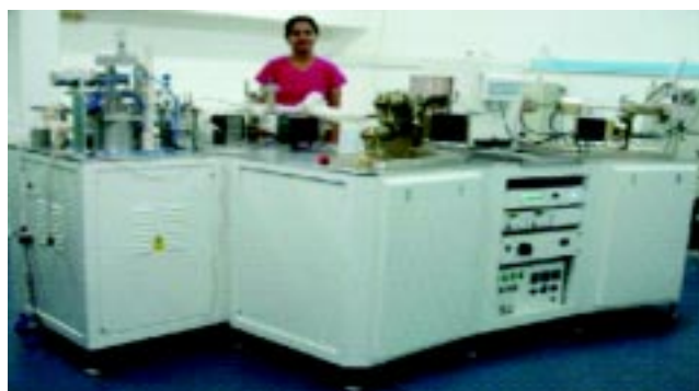
Fig. 31: Multi-collector noble gas mass spectrometer, recently installed at Thaltej, PRL.
