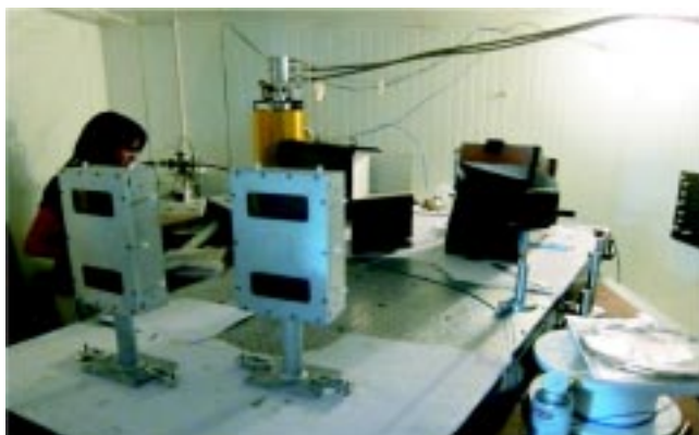
Fig.1:The Echelle Spectrograph installed in the inner Chamber.
