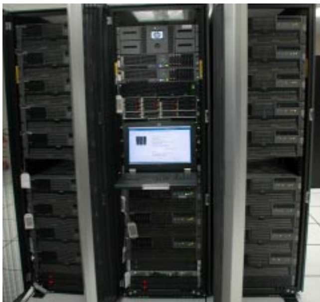
F&S.1: Twenty node cluster computer at PRL with a capacity to deliver 3 TFLOPS
