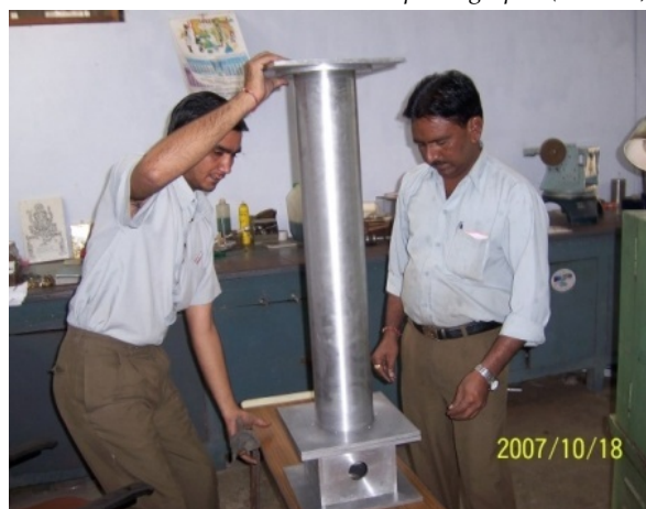
Figure 34 : Fabrication of Low Resolution Spectrograph in PRL workshop
