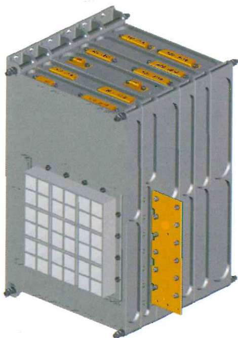
Fig. 5.1 : HEX detector package made up of six trays consisting of detector, front - end electronics, anticoincidence and power systems. Extra projection (Cu-coated) seen on the right hand side provides route for effective transfer of heat from the detector tray to a radiator plate for maintaining optimum temperature.
