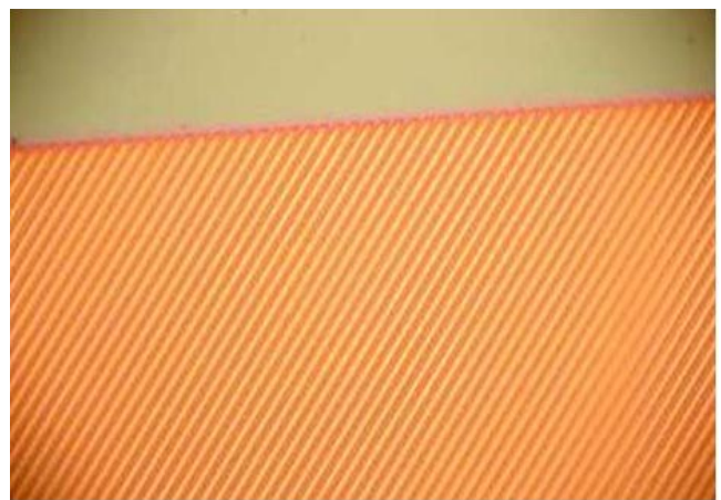
Fig. 3.3 : Photo-resist image of exposed grooves having SPD data with 100X. Step size is 0.01 microns
