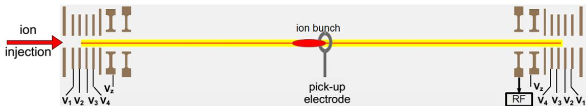
Figure: Schematic of the simulated Electrostatic Ion Beam Trap.
