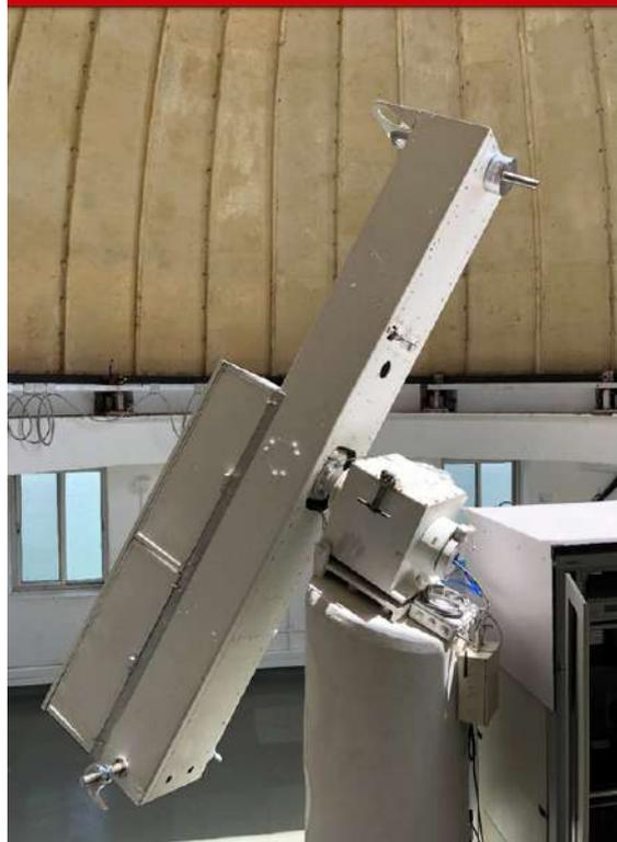
**Spar Telescope** : Till 2008, this telescope was used for high-resolution Observations in  $H\alpha$  with smaller FoV. From 2014 onwards this telescope is being used for full sun observations in three different wavelengths.
