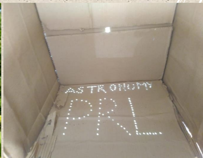
Figure : Images of the Sun during eclipse on 21 June 2020 made using pinhole camera
