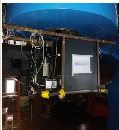
Fig 1: - MFOSC-P instrument mounted on PRL 1.2m telescope
