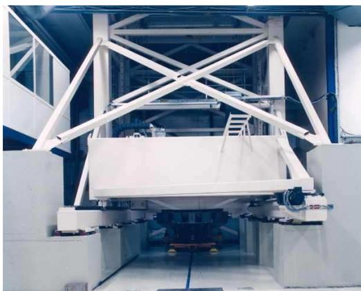
**AMOS Large Optical polishing facility with CCP process and interferometry test bench**
