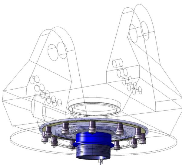
*Azimuth drive and Brakes*
