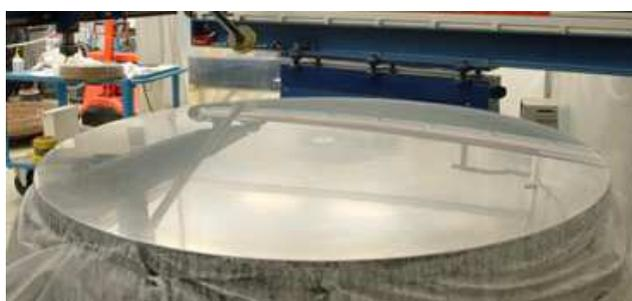
As part of the PLANCK Primary Reflector test bench, AMOS supplied to CSL a convex spherical mirror made of 5083 aluminium alloy.
