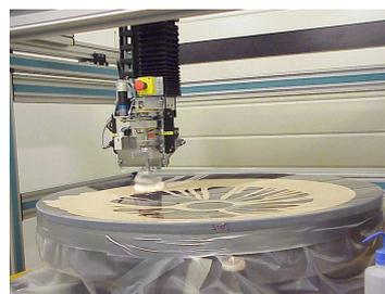
Ø an interferometry test tower (12 m height) with a movable platform equipped with a ZEISS interferometer DIRECT 100 and an holography test bench
