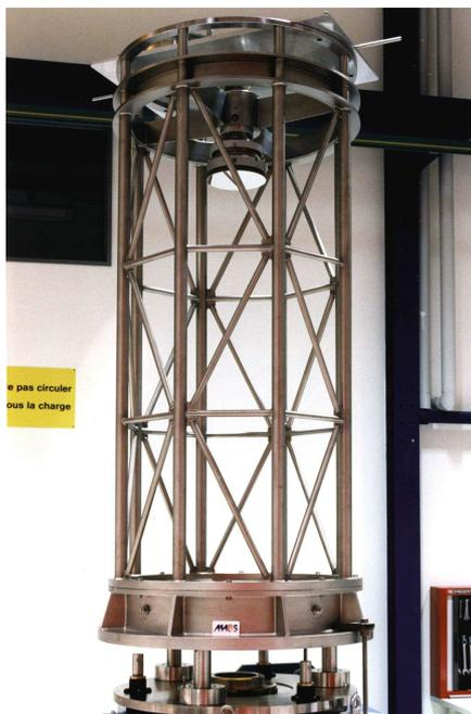
**EUV Collimator (800 mm Ø)**
