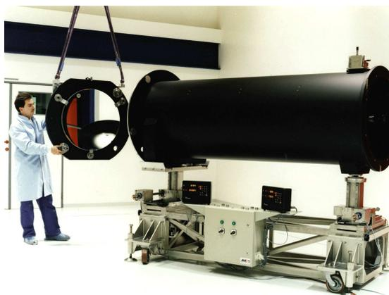
The ISO (Infrared Space Observatory) collimator is based on a Newton system with a parabolic primary mirror of 700 mm diameter and  $f/4$  aperture and a plane secondary which tilts the beam by 90 degrees. The wavefront error at 550 nm is smaller than  $\lambda/25$  RMS. The light sources are situated on the side of the tube and positioned by 3 crossed linear translation stages.
