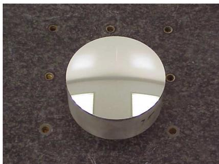
**mirror dia 75 radius 250: form: 11 nm RMS, Ra: < 2 nm**
