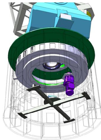
*View from bottom: Fold 5 and Motorized Cable Wrap*
