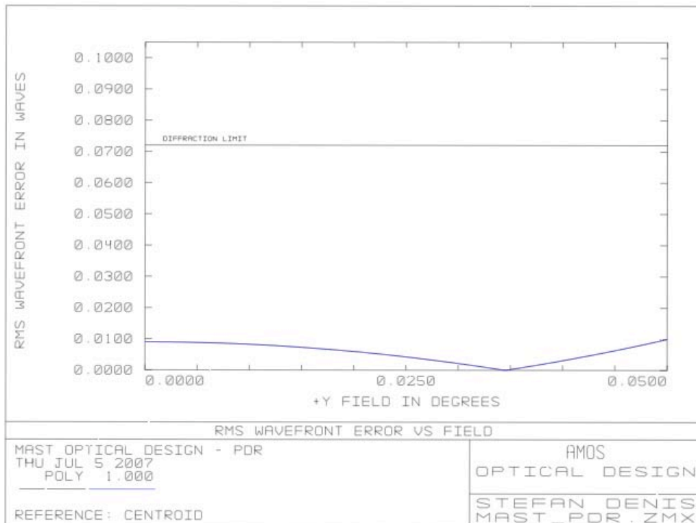
Figure 20: RMS WFE curve vs. FOV - with optimisation over FOV
