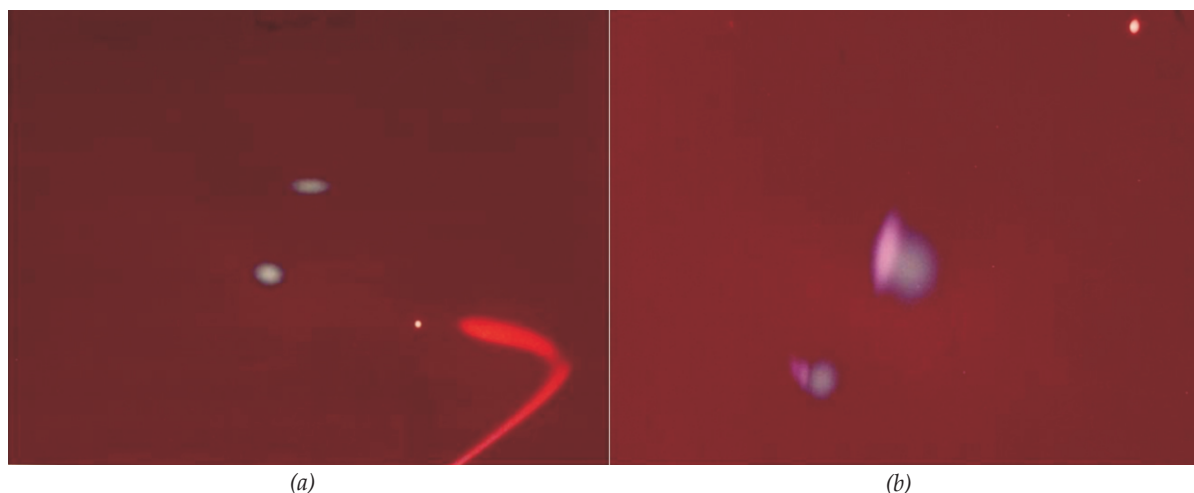
Fig.3: (a) Barium blob releases at altitudes of 137 and 150 km during upward leg and Lithium trail release which started from 132 km during downward leg of the Centaur rocket. (Launched from Thumba on 16 February 1980 at T_0 = 18:55 IST. This photograph was taken at T_0 + 755 seconds). (b) Barium blob released at altitudes of 183, 228 and 308 km. Rocket was launched from SHAR on 16 February 1982 at T_0 = 18:43:14 IST. This photograph was taken at T_0 + 305 seconds after the release of fifth blob. Third blob was released at T_0 + 123 sec. As can be seen from the figure Barium cloud is aligned with the magnetic field lines and Strontium which remains unionized is seen as a blob (R. Sekar, 1990, Ph.D. Thesis).
